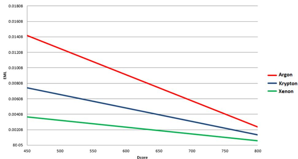
Figure 3: EML of argon, krypton and xenon for different Dcore at 1 THz for 6 μm strut width.
