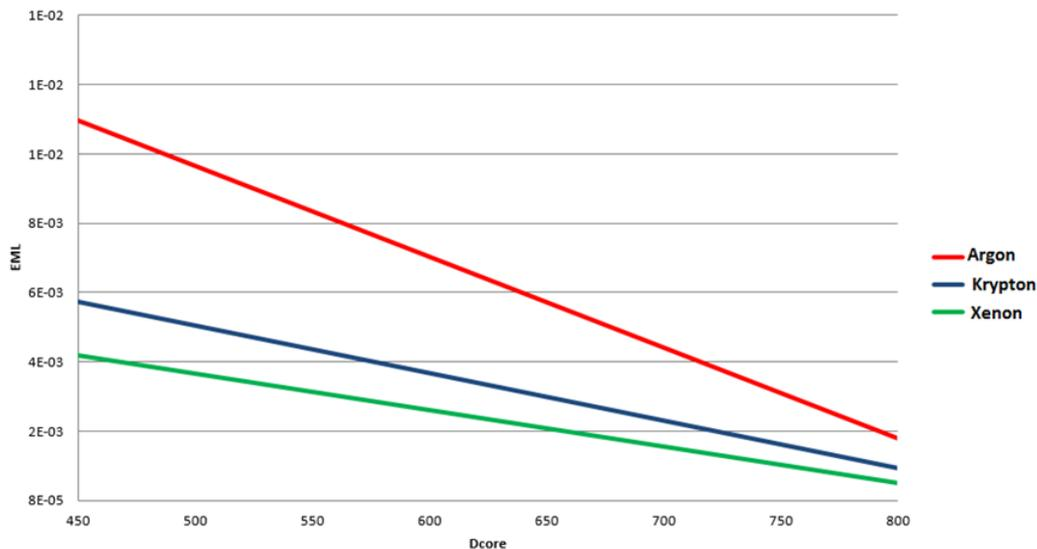
Figure 2: EML of argon, krypton and xenon for different Dcore at 1 THz for 5 μm strut width.
