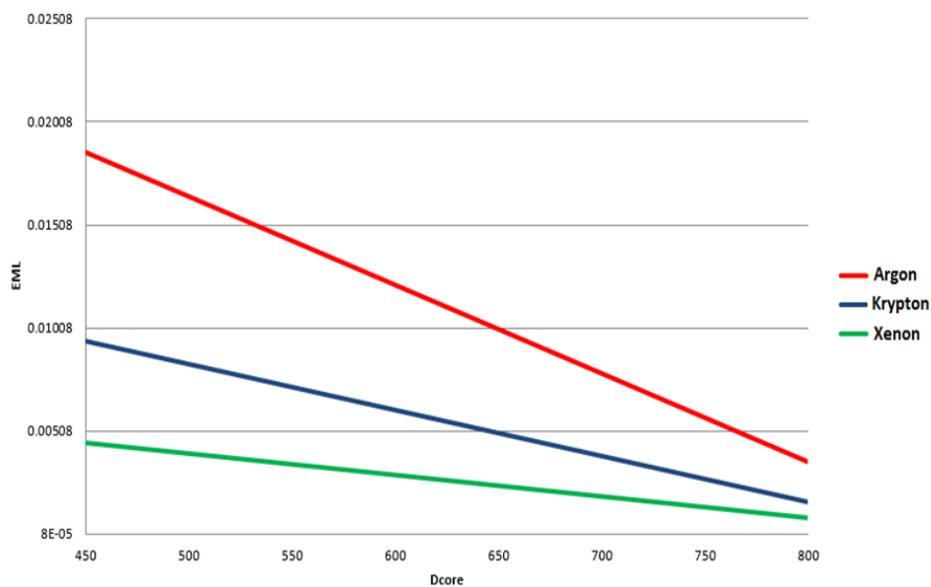
Figure 3: EML of argon, krypton and xenon for different Dcore at 1 THz for 7 μm strut width.
