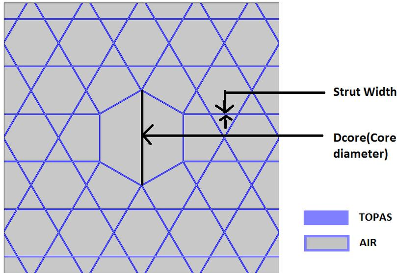
**Figure 1:** cross section of the hollow-core kagome lattice photonic crystal fiber
